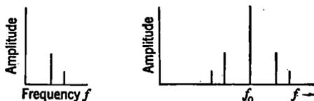
(a) Modulating function (b) Radio-frequency spectrum
